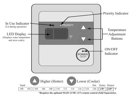
NOTICE: If the BATH control is turned on, the temperature setting on the MAIN control cannot be changed. The BATH control(s) will always have PRIORITY over the MAIN control.
